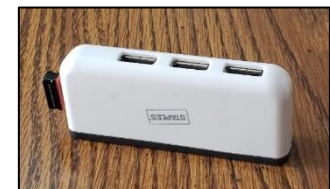
Fig. 12: Staples USB 4 port hub which allows more USB devices to be added
